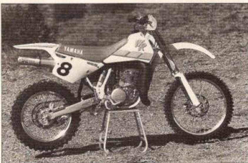
Yamaha fit our test bike with their YZ-R accessory spark arrester and hand guards to make the machine EPA-legal and better equipped to handle the tight stuff.
