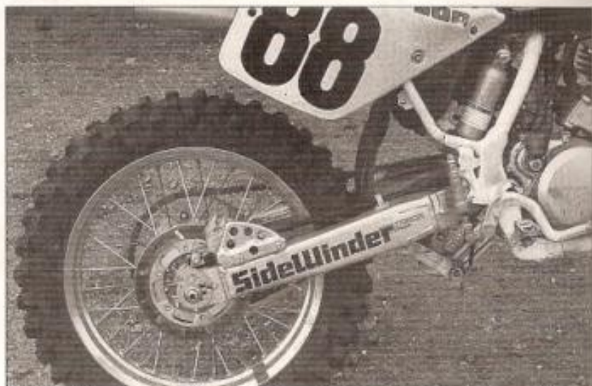
The rear brake is progressive and strong, yet not overly sensitive. The rear linkage hangs down low and can be a problem if you ride over big boulders or fallen trees.
