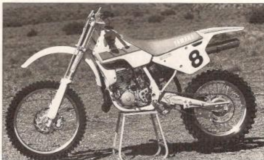
The new WR frame is similar to the 250's, yet is fit with all-new front suspension, a big tank, an 18-inch rear wheel and Bridgestone tires.
