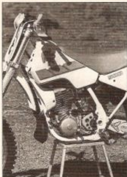
The WR's boost bottle is still hidden under the air shroud that directs a cool air flow to the finned cylinder. The tank looks great, but it's wide at the front and takes some getting used to.
