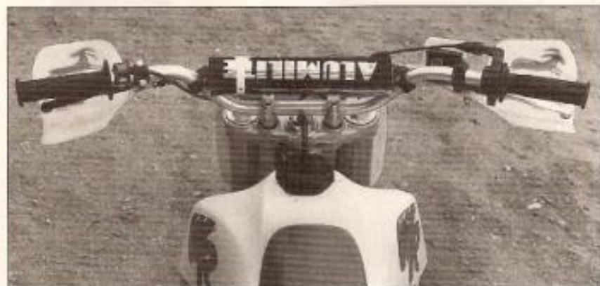
We shelved the stock handlebar and fit Answer's tallest Alumilite bar onto the machine. This modification helped dramatically when shifting from sitting to standing.
