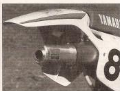
Yamaha's add-on spark arrestor bolts on easily and doesn't stifle the power. Good handholds are built right into the rear fender.
