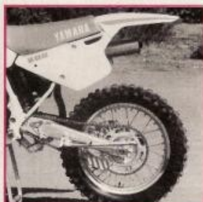
Yamaha's streamlined bodywork with integral lift handles appear on the 500, too, but the 500 also has a fully removable subframe and a swingarm-mounted kickstand.
