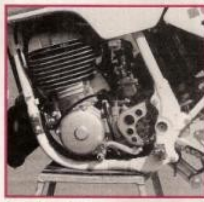
A smaller carb, lower compression and head mods update the reliable air-cooled power plant. The tank holds over three gallons, and the linkage matches the YZ250's but it works a shock with off-road valving.
