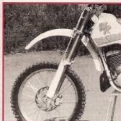
This is a fork that the YZ490 needed badly. Valved for a wider range of conditions than the motocross-only YZs, it features 43mm tubes, a cartridge design and fully adjustable damping.
